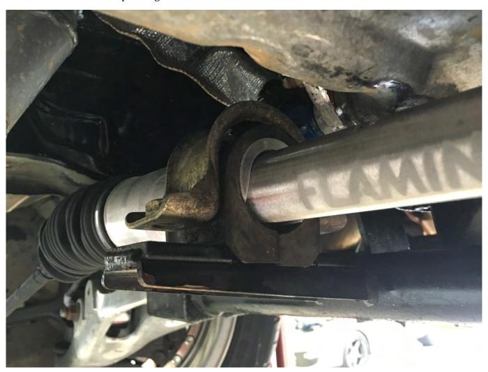
5 - Here is the drivers mount installed, U-BOLT CLAMP is used here now (older kit used weaker t-bolt)!
