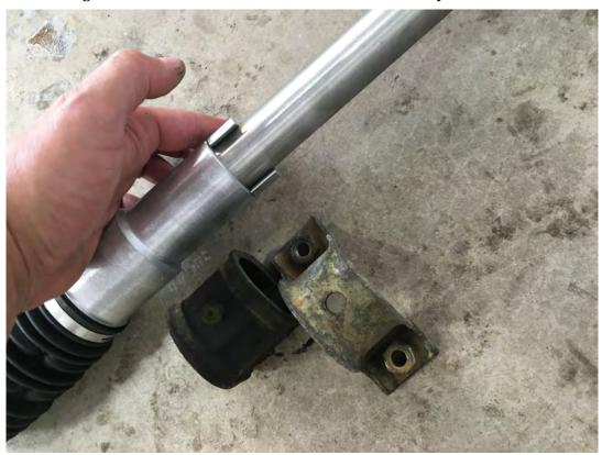
2 – Notice the hole in the drivers mount is facing towards the front side of the rack  $\,$
