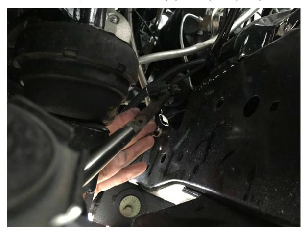
7 – Installed universal joint. Slide joint so it has good engagement on both splines.
