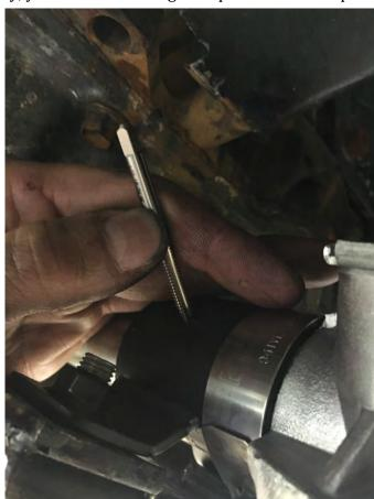
10 – Install the rotation locking bolt, do not overtighten!
