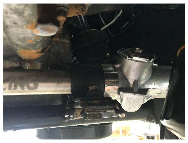
6 - Installed universal joint. Rotate rack to line up splines for good angle of operation.
