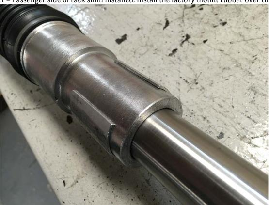
2 – Notice the hole in the mount is facing towards the front side of the rack. NOTE: THIS OLDER TBOLT STYLE CLAMP WAS WEAK. IT IS NOW REPLACED WITH STRONG U-BOLT CLAMP.
