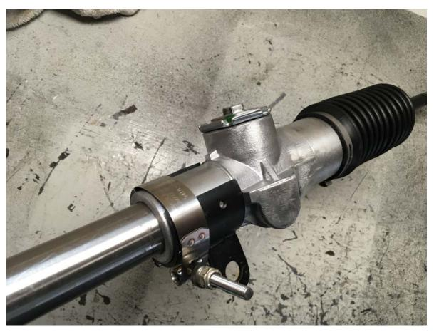
3 – Once you have rack installed and clocked properly, you will drill through the pilot hole and tap
