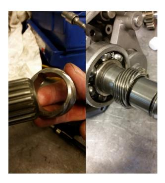
37. Install the locking ring on the other side of the speedo meter reader
