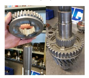
7. Install the bushing into the main shaft.
