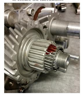
27. Install the 5<sup>th</sup> gear dog ring and the shift fork as a package
