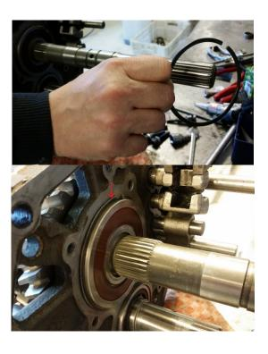
17. Install the bearing cover plate.
