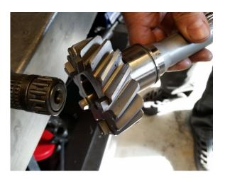
Then install the ½ gear shift fork and ¾ gear shift fork in the shift bar and tighten the screws. Remember to use the GREEN EXTRA STRONG locking glue! If the gearset is in rough use we even recommend to tack weld the shift fork bolts. Shift bars need to be moved towards the back of the transmissions to be able to install the shift forks.
