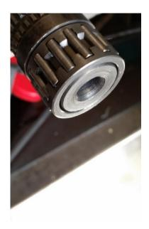
40. Install the input shaft bearing by heating it first to ensure the easy fitment (max. 120 degrees Celsius).
