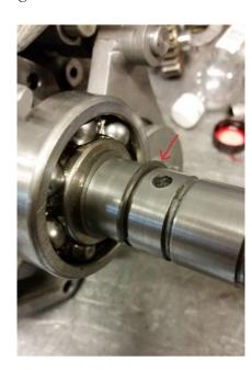
35. Install the speedo meter reader locking ball in the main shaft hole.
