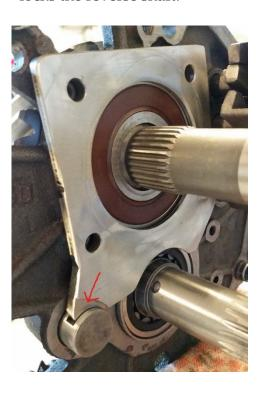
18. Install the 5<sup>th</sup> gear sprocket on the main shaft until the center plate bearing. Please, check that it will be installed the correct side facing the bearing.
