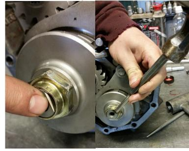
31. Install the socket on the main shaft \*HD\*
