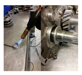
22. Install the oil bushing on the counter shaft.
