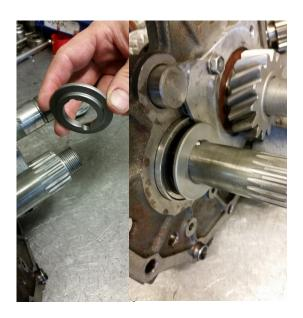
21. Install the counter shaft 5<sup>th</sup> gear bearing bushing. Remember to heat it well (maximum 120 degrees Celsius) before installing it to confirm it goes to it's place without needing to use any force.
