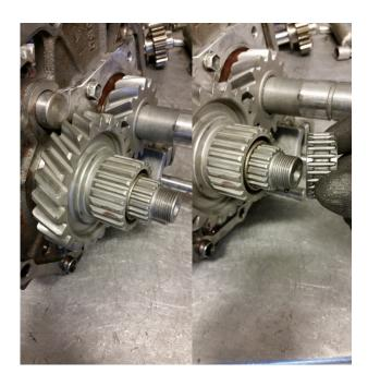
24. Install the 5<sup>th</sup> gear counter shaft needle bearing
