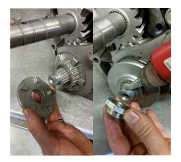
30. Hit the corner of the nut by using a hammer until it touches the flat part of the counter shaft end to secure that the nut doesn't come off by accident.
