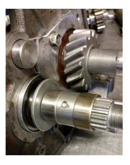
25. Install the 5<sup>th</sup> gear sprocket into the counter shaft.Install the 5<sup>th</sup> gear needle bearing
