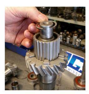
3. Install the 2<sup>nd</sup> gear needle bearing in the main shaft from the rear side. Remember to put some transmission oil around it to ensure the lubrication
