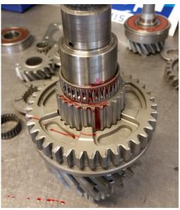
10. Install the needle bearing for the 1st gear sprocket
