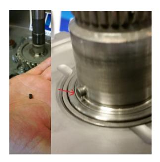
12. Install the 1<sup>st</sup> gear thrust washer Please, check the photo carefully to install the thrust washer the correct way. \*HD\*
