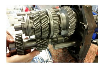
16. Install the center plate bearing locking ring. Make sure it'll drop into the groove.
