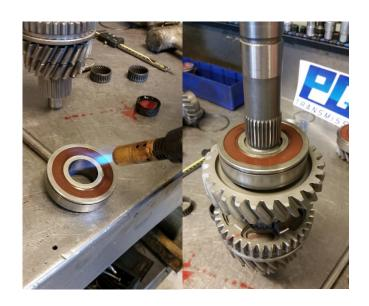
15. Install both shafts in the center plate (from the front side). They must be installed together. Be careful not the harm the center plate bearings.\*HD\*
