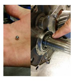
20. Install the 5<sup>th</sup> gear thrust washer bearing so that the ball locks it.
