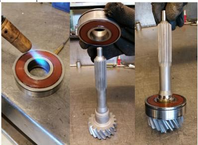
41. Install the input shaft. Input shaft can be also installed after the casing is already installed. The input shaft bearing should have been installed at this point but is missing from this particular photo.
