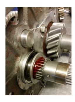
26. Install the 5<sup>th</sup> gear needle bearing inside the sprocket and remember to put some transmission oil on it to ensure the lubrication.
