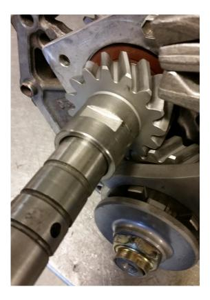
33. Install the locking ring into the groove next to the bearing to lock the bearing.
