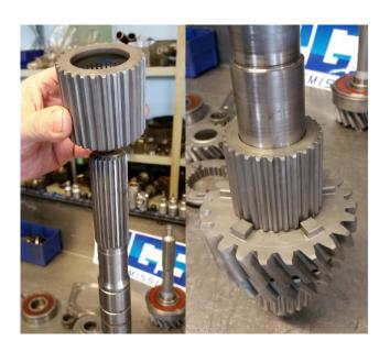
6. Install the 1-2 gear dog ring / main shaft reverse gear sprocket.
