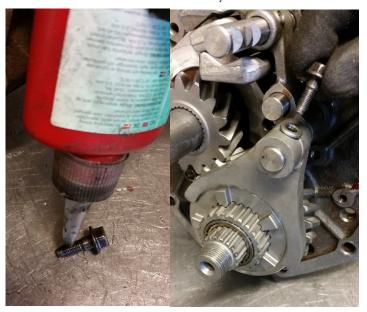
29. Install the 5<sup>th</sup> gear dog plate and the nut. Use screw locking glue for securing the nut.
