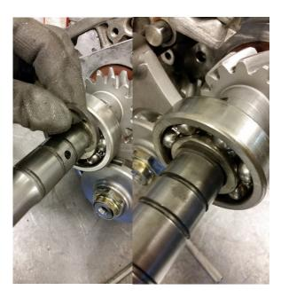
32. Install the bearing until it touches the socket. Remember to heat it with a heater (max. 120 degrees Celsius) to ensure it will fit in it's place without force needed.
