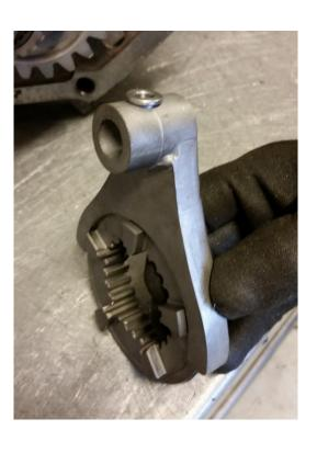
28. Install the shift fork / dogring package on the counter shaft on the 5<sup>th</sup> gear sprocket and install the screw and tighten it into the 5<sup>th</sup> gear shift bar. \*HD\* Remember to use the GREEN EXTRA STRONG screw locking glue!! We even recommend to tack weld the bolt to the shift fork to fully secure it.
