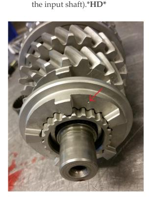
13. Heat the center plate bearing with a heater (maximum 120 degrees Celsius) so that it'll fit easily through the main shaft until the thrust washer bearing.
